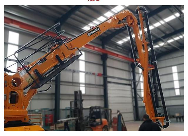
Featuring a compact structure, the Atlantic Concrete Placing Boom can be lifted and transferred to any suitable place for concrete placement, such as floors, platforms, simply-structured racks or even trailers.
